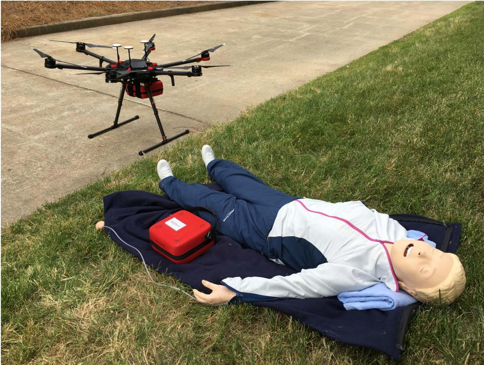
**Supplementary Figure S1.** DJI Model M600 drone fitted with AED and Laerdal Resusci Anne at simulated cardiac arrest event site.
